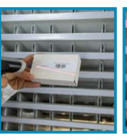
Drugs are quickly and safely intro- Take into account that picking and duced into the channels, thanks to «Stock to light Sentinel» technology, on the back side of the machine. Led lights guide the operator to the right drug location.
