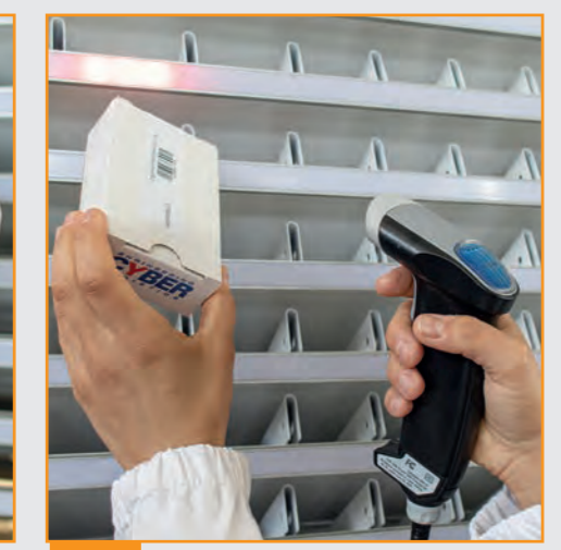
B Insertion of the package in the correct storage channel indicated by the red led light.
